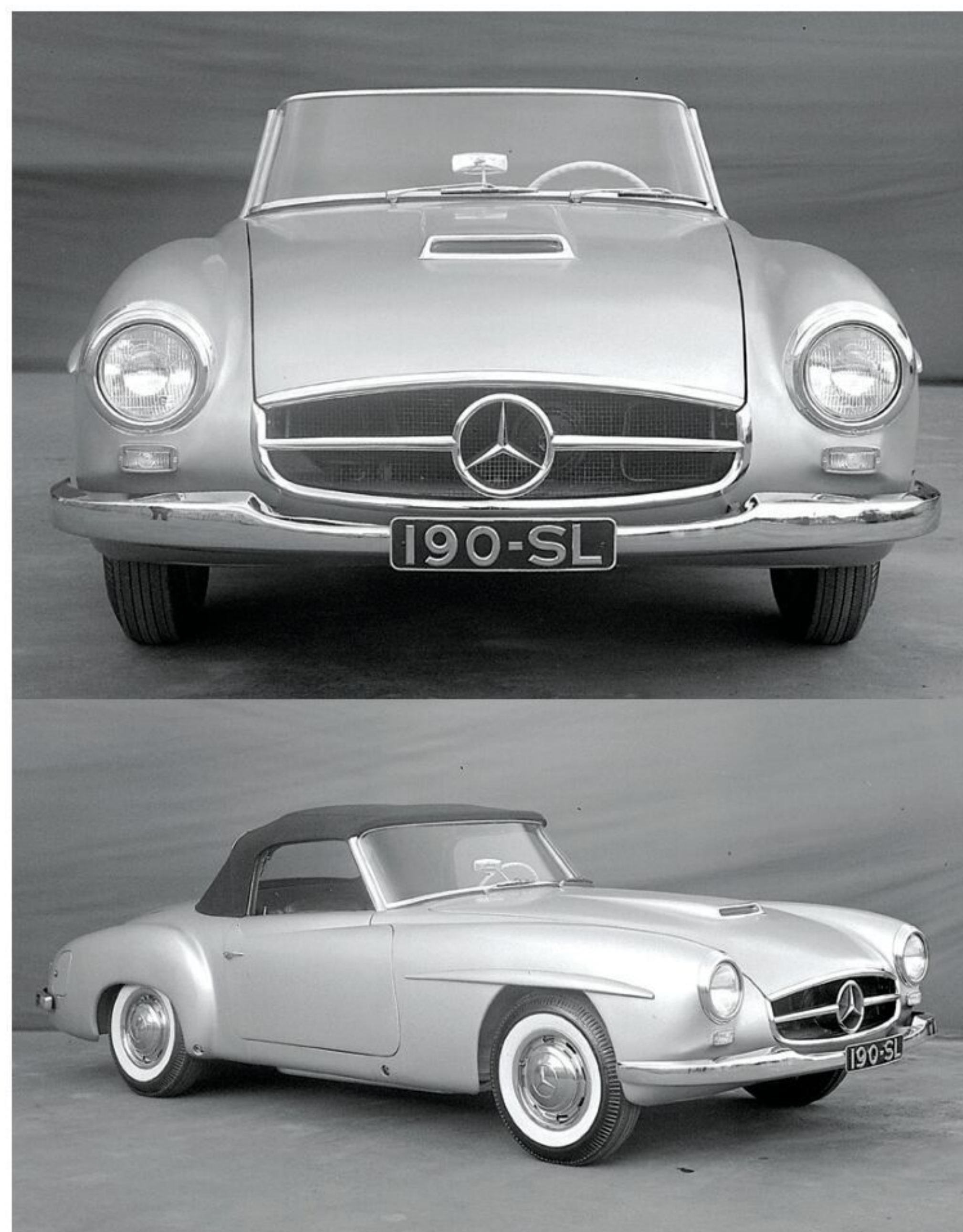
Above Pre production car featured an air intake in the centre of its bonnet.
