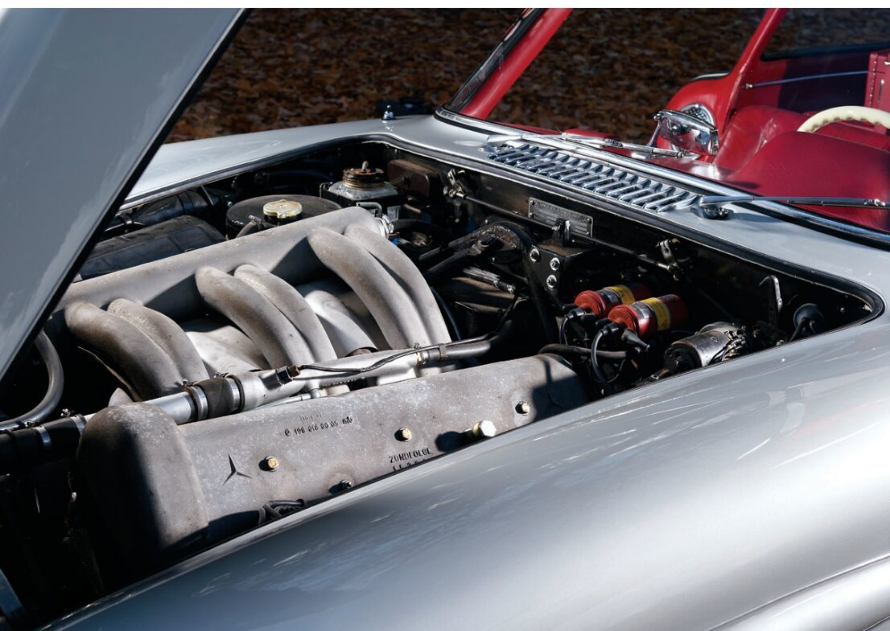
Left Fuel injected M198 motor at a 45-degree angle.
