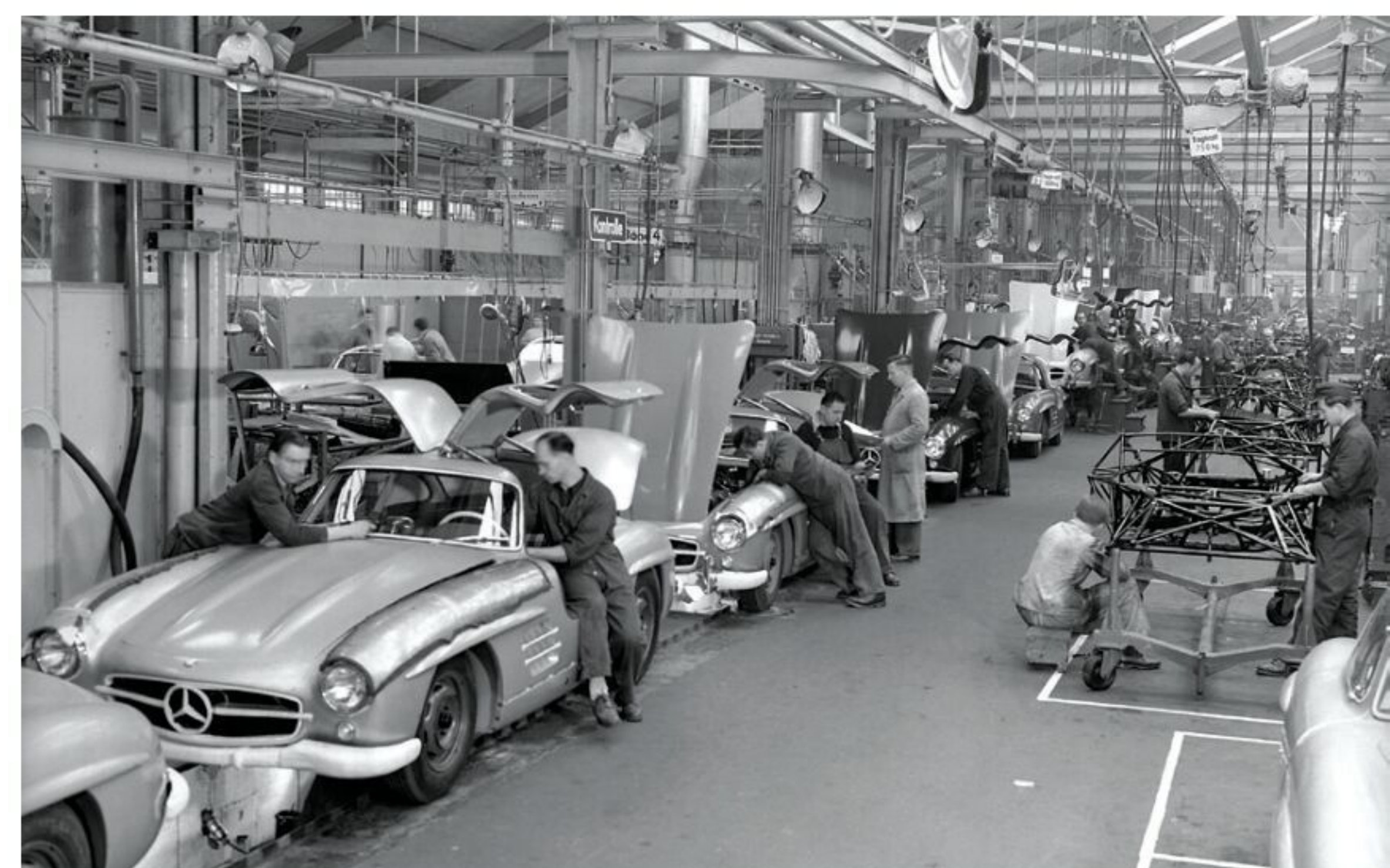
Right and far right Sindelfingen line in 1955; lightweight space frame chassis.
