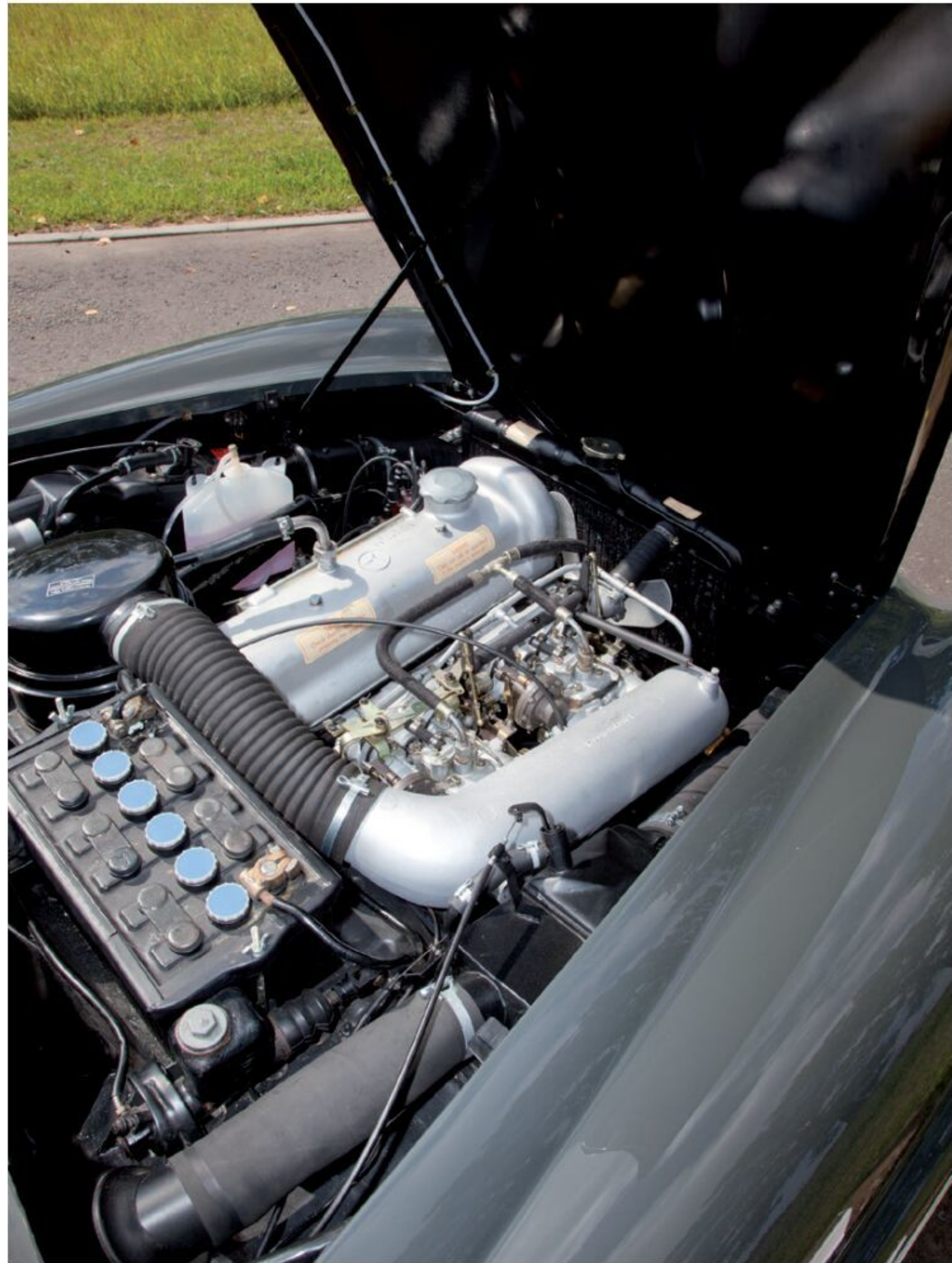
Above Four-cylinder motor with a pair of Solex 44 PHH carbs.
