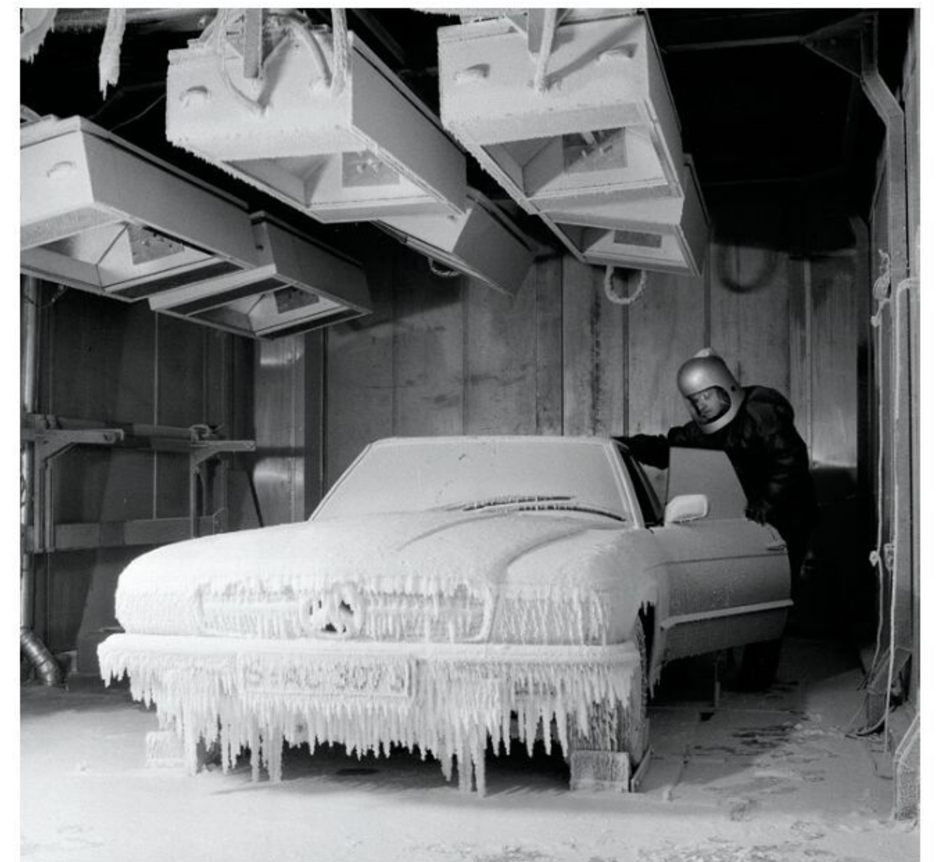
Above 350SL testing on a dynamometer at -25C in a cold chamber.
