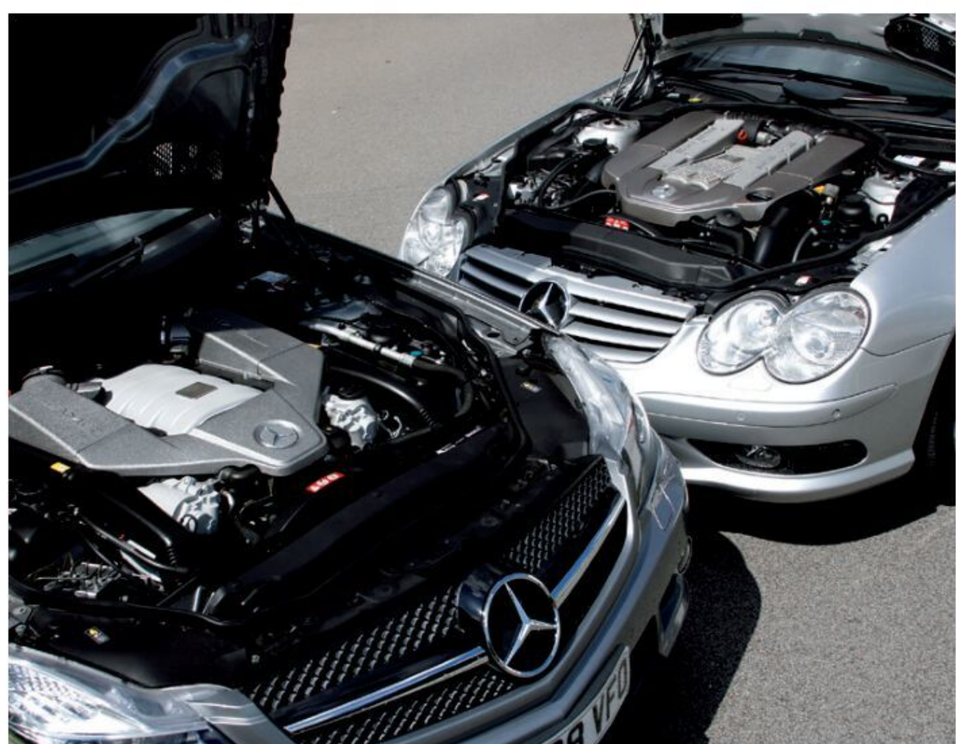
Left 6.2-litre V8 replaced 5.4-litre V8 Kompressor in 2008.
