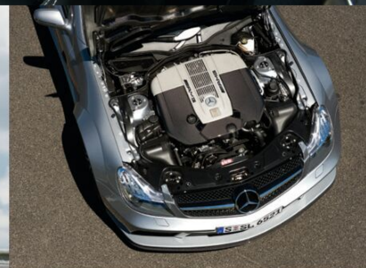
Above SL65 AMG Black Series packed a 661bhp V12 unit.
