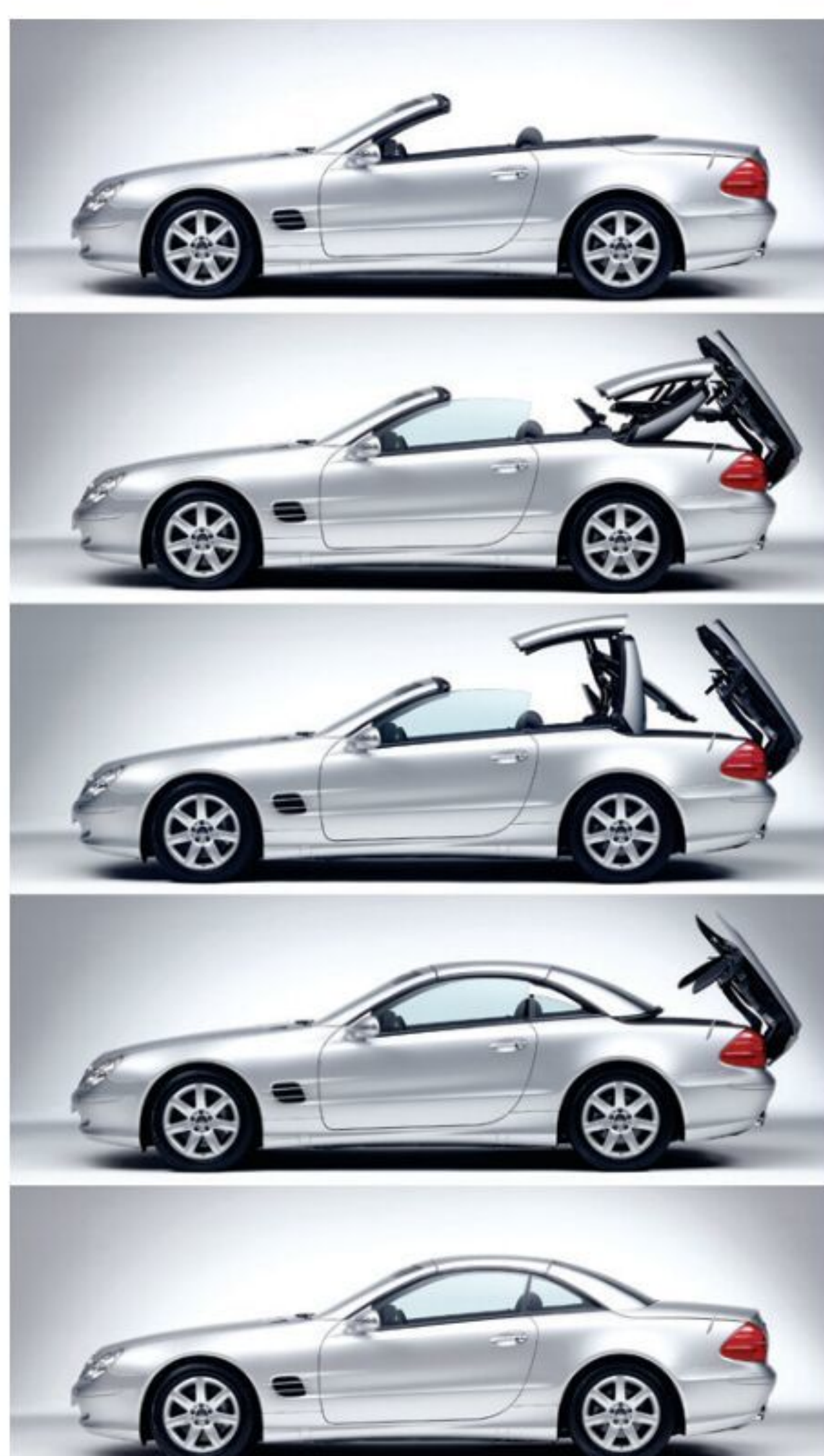
Above Press a button on the centre console and the SL goes from roadster to coupe.
