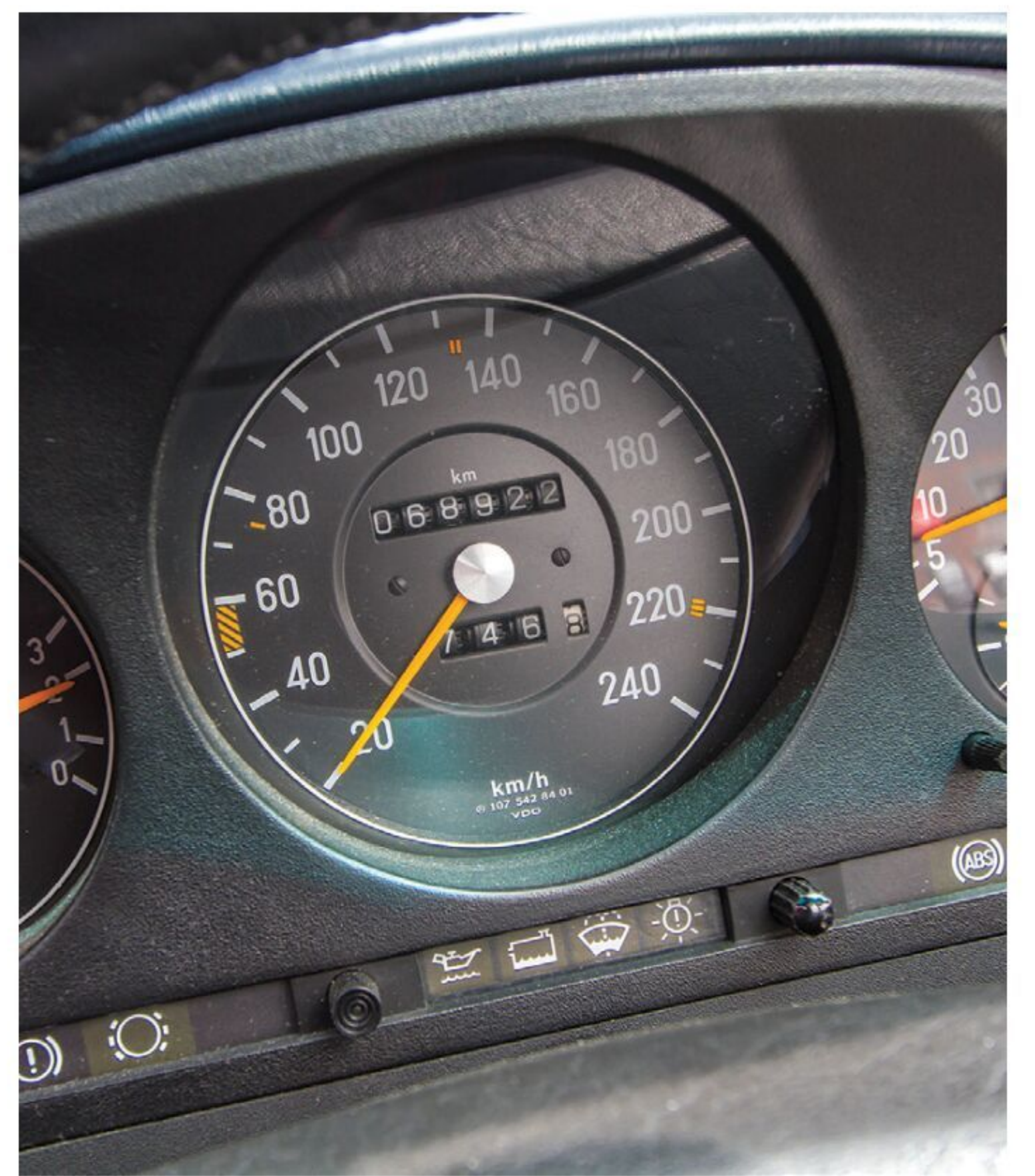
Above Speedometer with marks for max speed in each gear.
