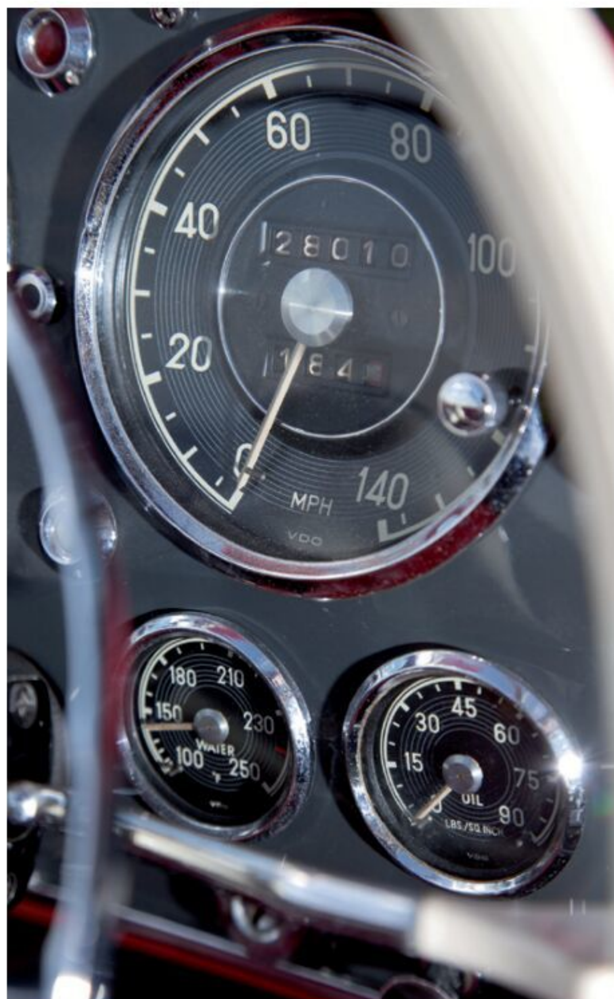
Above Speedo, water temp and oil pressure gauges with chrome surrounds.
